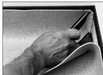
3. Fold in one side and gradually cut off the surplus material to complete the first part of the corner.
