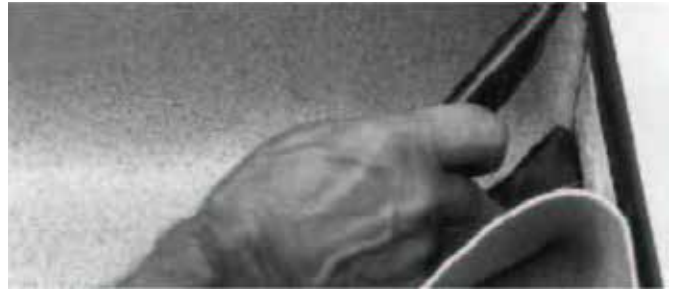
3. Fold in one side of the mitre and carefully cut off the surplus material.
