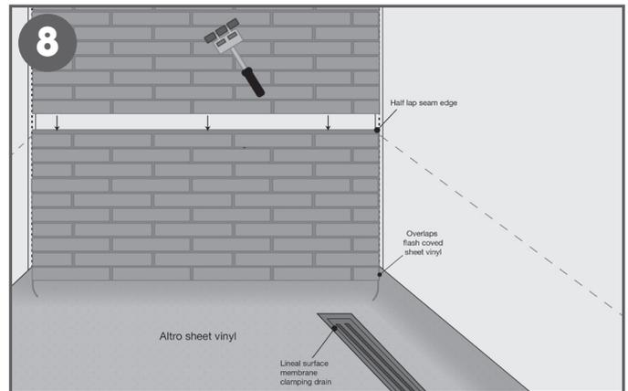
8. Install the top panel as previously instructed with correct space and properly aligned with the previously installed bottom panel. Use a 3-wheeled wall roller to roll entire panel to ensure proper bond to wall substrate.
