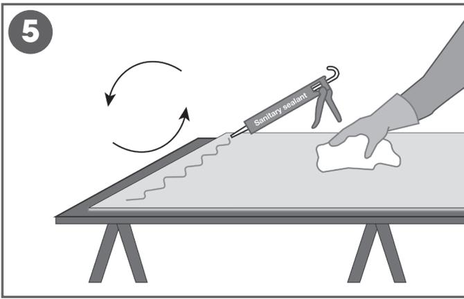
5. Clean the back of the panels to remove dust and contaminants. Apply Altro sanitary sealant on the back of the panel where it will overlap the existing covered flooring.
