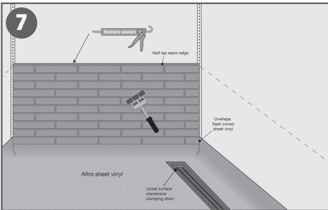
7. Install panel into position with correct spacing and aligned on or with datum line. Use a 3-wheeled wall roller to roll entire panel to ensure proper bond to wall substrate. Apply a 2mm bead of Altro sanitary sealant to the half-lap seam edge. Be sure to keep it above the visible seam edge.
