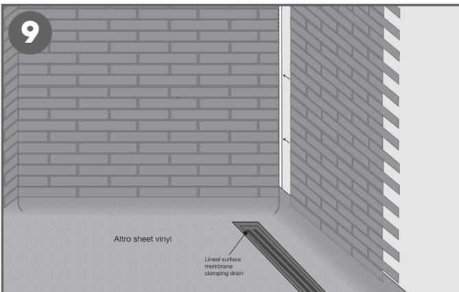
9. Additional wall panels that are not in direct contact with continuous moisture can be installed vertically with the interlocking joining method. This allows full panels to be installed without any horizontal seams. Install adjacent panels as previously instructed.
