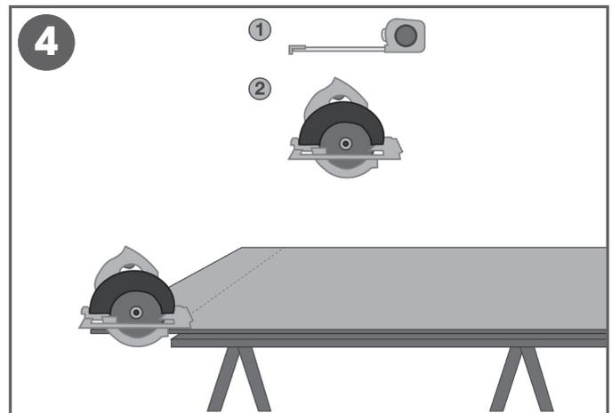
4. Measure and mark out the previously determined measurements onto the panel. Make necessary cuts. Always dry fit to ensure proper fit.
