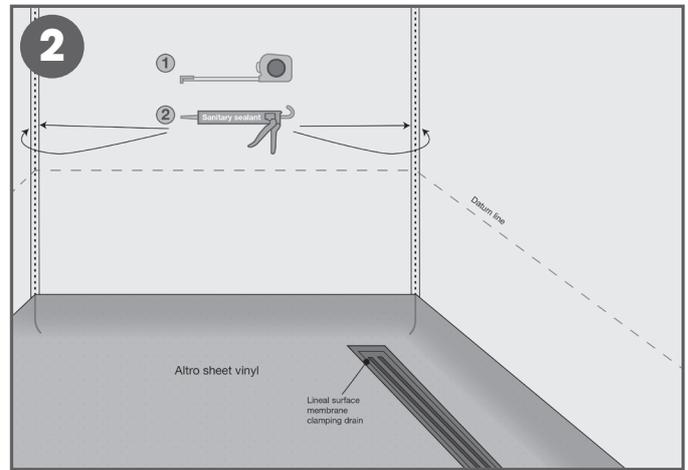
2. Apply a bead of Altro sanitary sealant to the substrate vertically on both sides of the corner where the sheets are to be installed.
